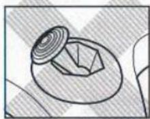
If the Control Stick is held at an angled position (as shown in the picture on the left) when the power is turned ON, this position will set as neutral. This will cause games using the Control Stick to operate incorrectly.
